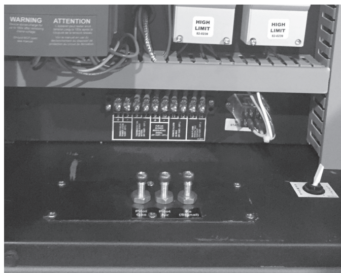
Figure 16 Manometer connections to the test manifold (in control cabinet)
